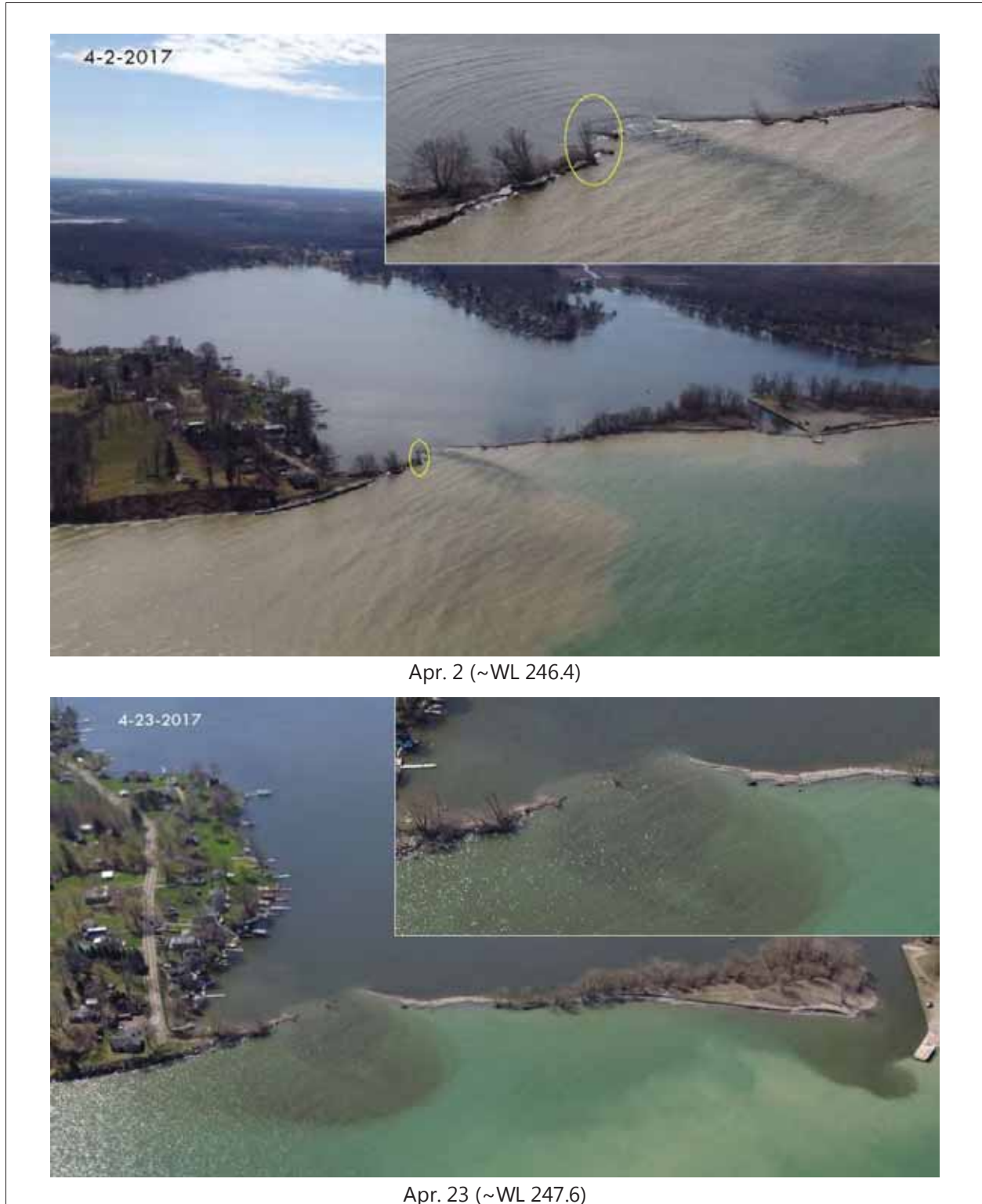
Figure 2.1-12 Port Bay and East Barrier Bar Breach, April 2017 (aerial view)
