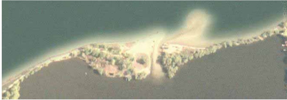
Deflection of LST due to the pier and channel flow, Oct. 11, 2008
